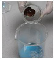
**5.** Add about 10 mL of distilled water to the solid copper and swirl to wash any remaining ions from the copper. Decant the wash water from the copper and add 10 more mL of distilled water, swirl and decant again. Wash copper particles finally with several mL of acetone (**CAUTION**-Acetone is very flammable). Swirl and allow standing a few minutes. Decant off the acetone.
