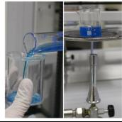
**3.** Slowly add hot  $CuSO_4$  solution to the beaker that contains the iron powder. Stir the mixture a few times until completeness of the reaction. You should see copper forming. When the reaction has finished, allow the copper product to cool.
