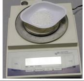
**3.** Immediately, add the weighed amount of salt, swirl to dissolve (use stirring rod if necessary), and continue taking temperature data at 30 seconds intervals.
