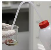
**6.** The acetone readily dissolves the water and helps the removal of it from the medium. Swirl the beaker gently on low heat flame. Copper product should be spread in a single layer on the bottom of the beaker. Grinding of aggregates with a spatula makes the copper easy to dry. Be sure not to remove any copper from the beaker.
