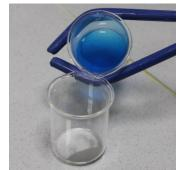
**4.** Then carefully decant the liquid from the copper into the waste container. Be careful not to lose any copper.
